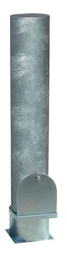
Wembley model bollard made of hot-dip galvanized steel tube with a diameter of ø 100, 120, 168, 220 mm. and a thickness of 3 mm. Total height of 1000 mm.
